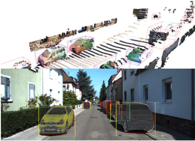
Fig. 9. Automatic generation of 3D object detection labels via rendering by Zakharov et al. [46] (upper) and Beker et al. [125] (lower).
