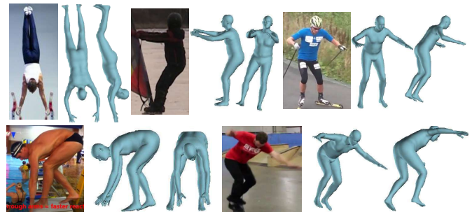
Fig. 7. Human body estimation trained with silhouette and keypoint supervision by Pavlakos et al. [10].
