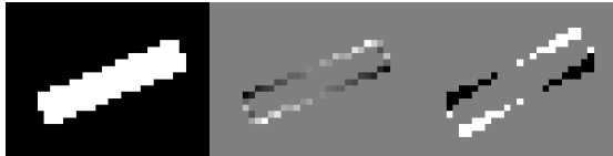
Fig. 7. Differentiable rendering versus finite differencing. Left: a rotating quadrilateral. Middle: OpenDR's predicted change in pixel values with respect to in-plane rotation. Right: finite differences recorded with a change to in-plane rotation.
